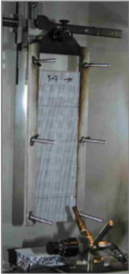
Figure 5.5: Picture of sample about to undergo ISO 11925-2 test
