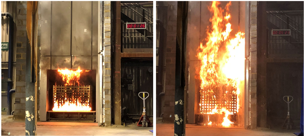
Figure 5.9: photographs of a BS 8414 test in operation
