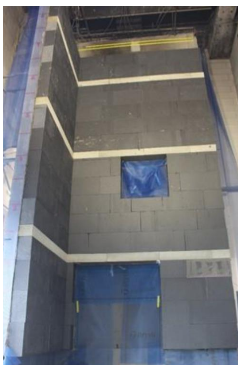
Figure 4.5. Specimen is under construction at the laboratory of MFPA.
